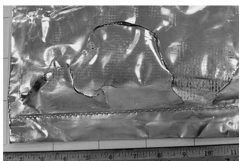
Fig. 2 Through-thickness cracks in 5-mil Al-FEP outer layer MLI from bay 10, photographed after retrieval during SM3A.
